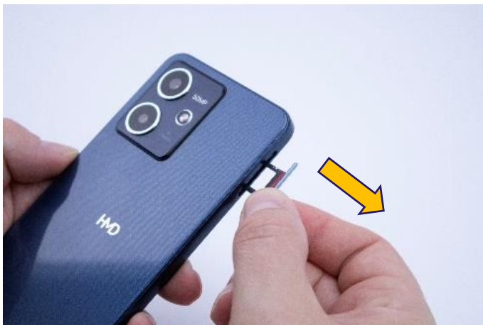
Insert opening tool SRT6
