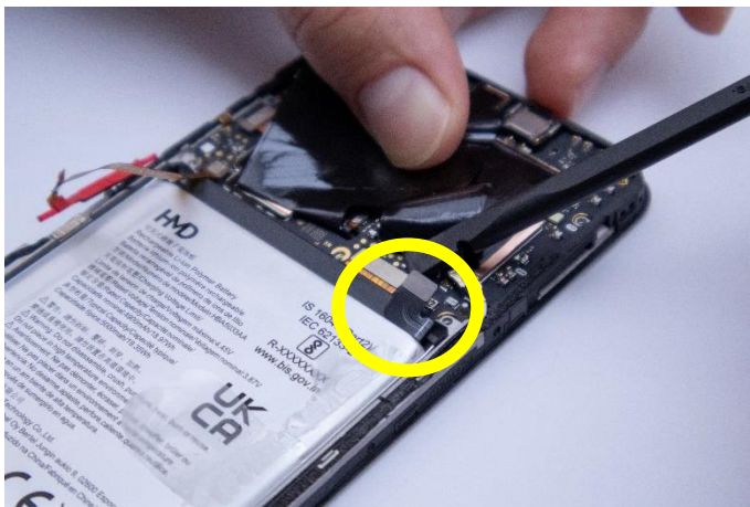
Disconnect main flex cable
