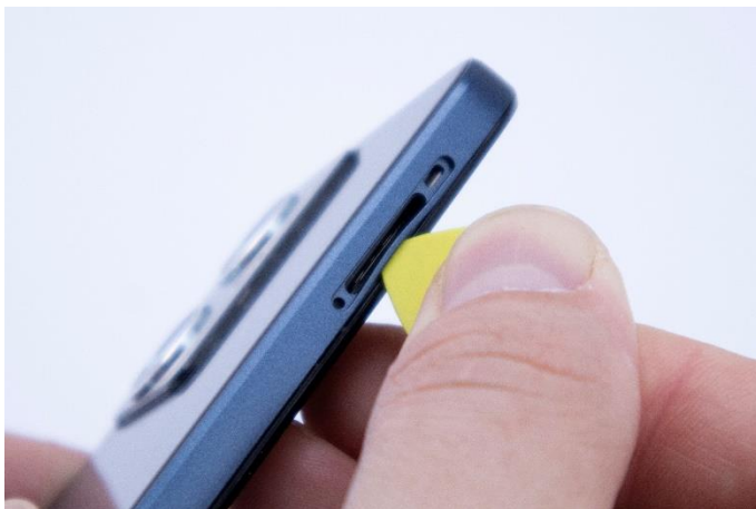
Insert opening tool SRT6
