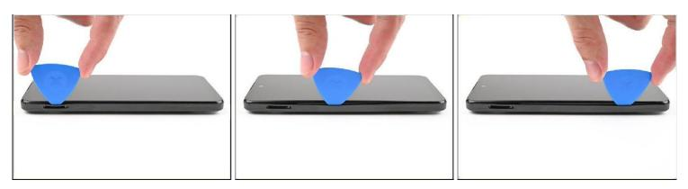
$^ullet$  Slide the opening pick along the left edge to begin unclipping the back cover.
