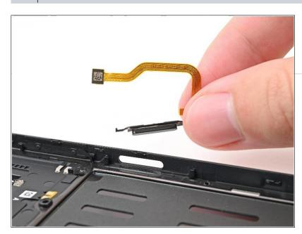
• Lift the power button out of the recess in the back cover and remove it.
