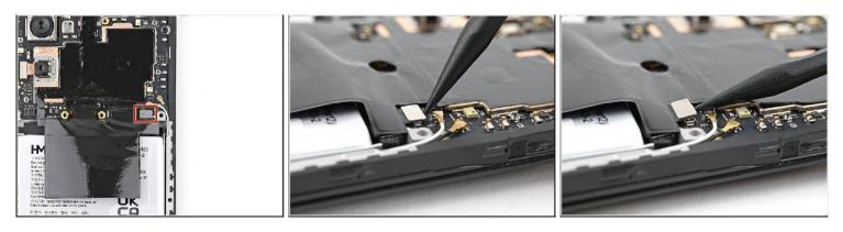
• Use a Spudger to pry up and disconnect the battery press connector. (Refer Snap -1 onnext Page )
