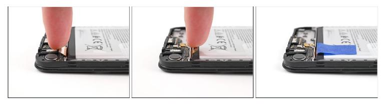
• Move the interconnect cable press connector toward the battery to keep it out of the way of the charging board in the next step.
