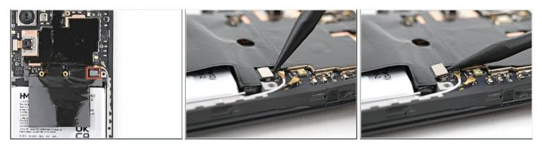
Use a spudger to pry up and disconnect the battery press connector. (Refer Snap-1 on
