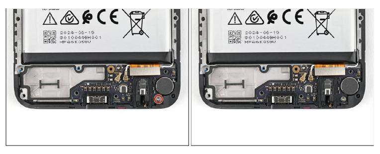
Use a T3 Torx screwdriver to remove the 3.3 mm-long screw securing the charging board.
