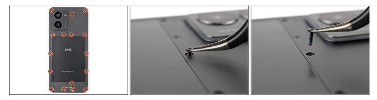
Use a T3 Torx screwdriver to remove the sixteen 5.0 mm-long screws securing the
