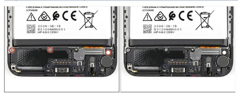
A Be careful not to puncture or damage the battery with your tool during the rest of this guide.
