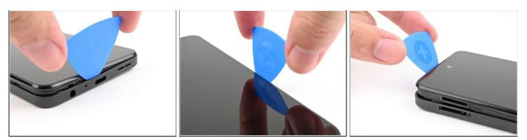
• Continue sliding the pick around the perimeter of your phone until the back cover is fully
