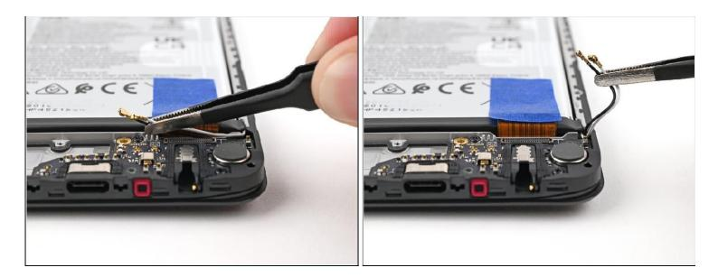
• Use tweezers, or your fingers, to move the two antenna cables out of their slots near the
