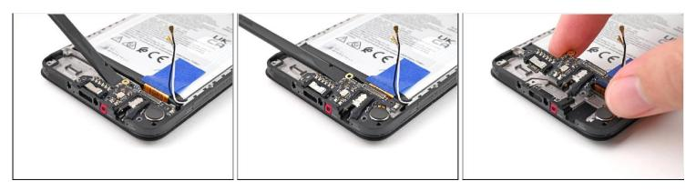
Lift the charging board out of the frame and remove it.
