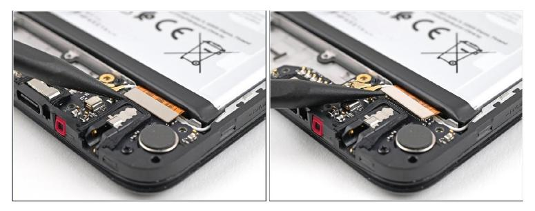
• Use a spudger to pry up and disconnect the interconnect cable press connector.
