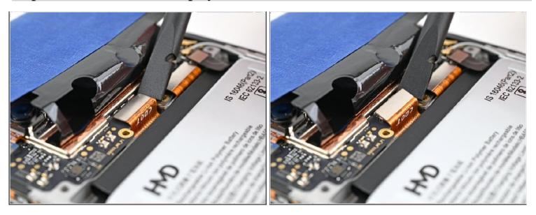
$^ullet$  Use a spudger to pry up and disconnect the display press connector.
