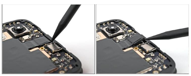
Use the tip of a spudger to pry up the front camera from the frame and separate its adhesive.
