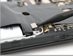
Use a spudger to pry up and disconnect the battery press connector (Refer Snap-1 on lastPage).
