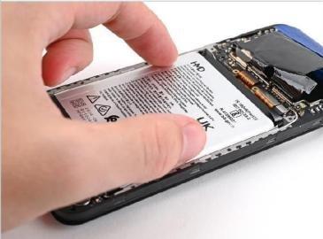
• Firmly press the battery into its recess to secure it with the adhesive.
