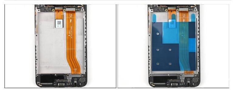
Align the new battery adhesive over the frame, making sure that the three adhesive strips overlap properly.
