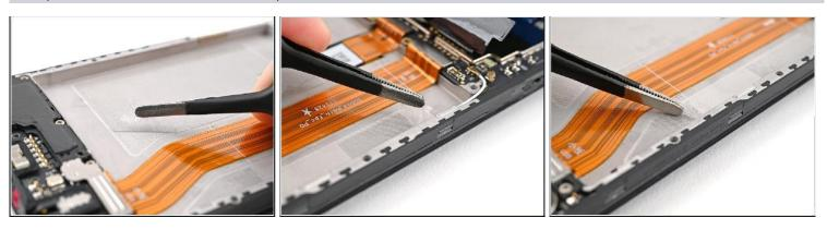
• Use tweezers, or your fingers, to peel the three battery adhesive strips off the frame.
