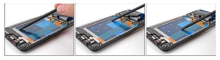
• Use the flat end of a spudger or your fingers to press the adhesive onto the frame.
