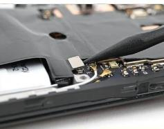
Use a spudger to pry up and disconnect the battery press connector (Refer Snap -1 on next Page).
