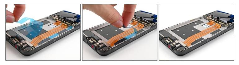
• Remove the two remaining liners to expose the adhesive.
