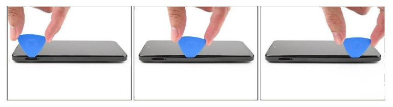
• Slide the opening pick along the left edge to begin unclipping the back cover.
