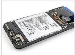
While holding the battery over its recess, temporarily reconnect the battery connector.
